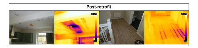
Figure 33. Air infiltration (under dwelling depressurisation at the post-retrofit stage) passing through the intermediate floor void and emerging on the landing.
