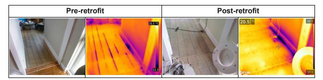
Figure 32. Air infiltration (under dwelling depressurisation) at the lounge floor before and after retrofit.
